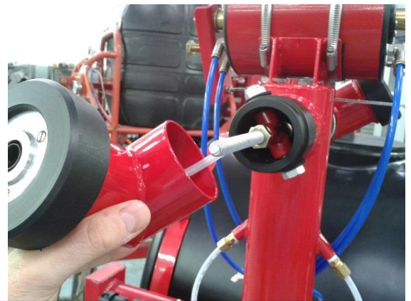
The barrels are linked together from the inside in order to turn simultaneously when the reversion is switched on or off.
