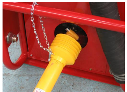
Correct mounting of the driveshaft. Fix chains to prevent guard from rotating!
