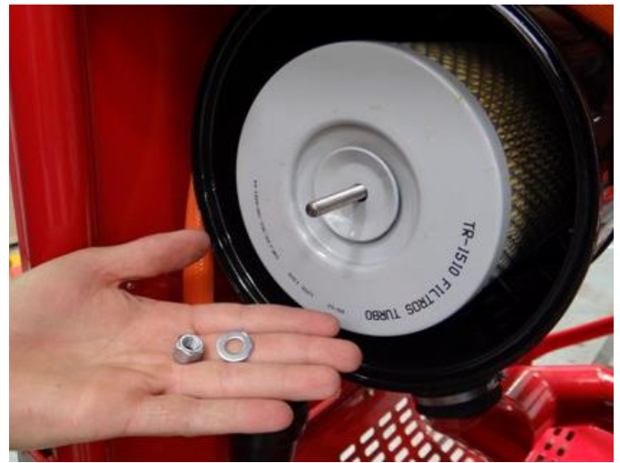
To remove element release nut.
