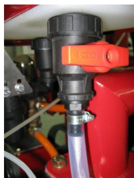
Drain valve (shut)
