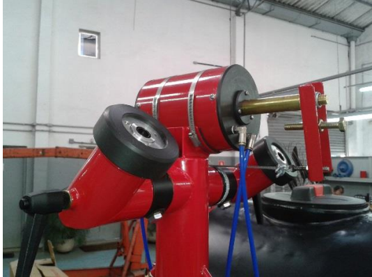
Nozzles may be pointed to left side or right side of tractor's motion.
