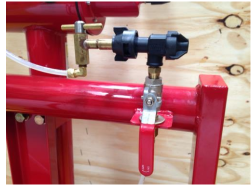
One of two anti-drip valves on the TracFOG 100 F
