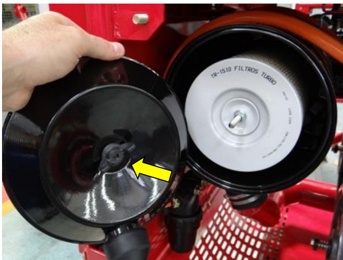
To open filter release butterfly nut.
