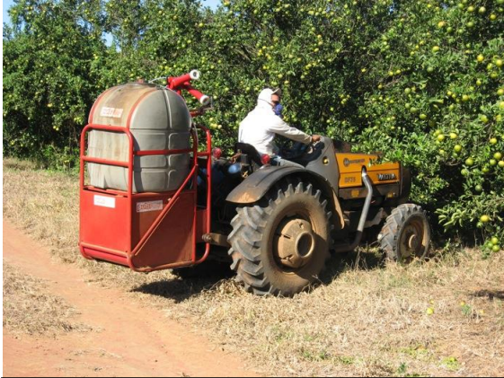
The unit should be leveled when lifted about 20-50 cm, depending on tractor size.
