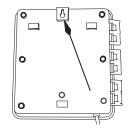
center location to mark position for second anchor. Remove controller from top keyhole and install second anchor and then remount controller and tighten both screws to secure unit.
