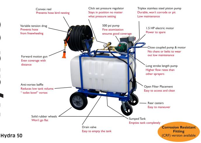
The Dramm Hydra Multi-spray Hydraulic Sprayer is a high volume hydraulic sprayer capable of performing a variety of tasks. The Hydra is perfect for the application of insecticides, fungicides, growth regulators, fertilizers, disinfectants and other chemicals.
